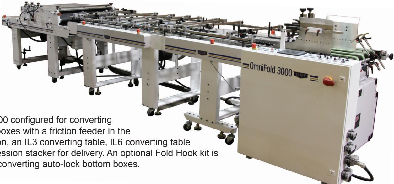
OmniFold 3000 configured for converting cartons and boxes with a friction feeder in the docking station, an IL3 converting table, IL6 converting table and a compression stacker for delivery. An optional Fold Hook kit is available for converting auto-lock bottom boxes.
